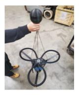
**Optional:** connect rope to three arms of diffuser for easier retrieval.
