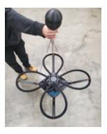
**Optional:** connect rope to four arms of diffuser for easier retrieval.
