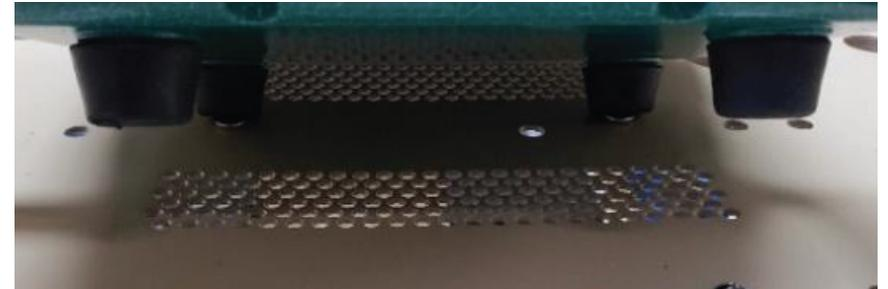
Guide the sinking airline from the manifold through the holes to outside of the cabinet.
