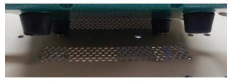
Guide the sinking airline from the manifold through the holes to outside of the cabinet.
