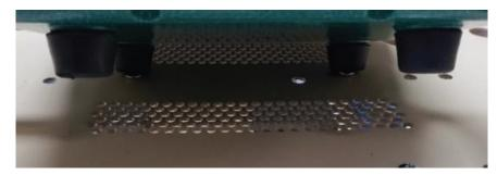
Guide the sinking airline from the compressor through the holes to outside of the cabinet.
